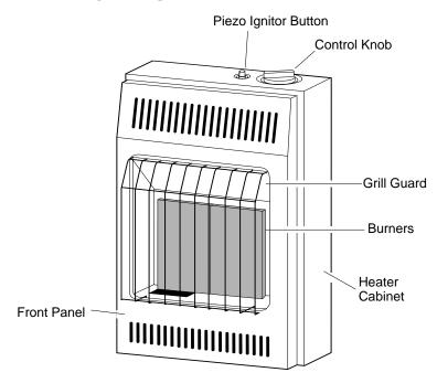
Figure 1 - Vent-Free Natural Gas Heater (Model VN10 Shown)
